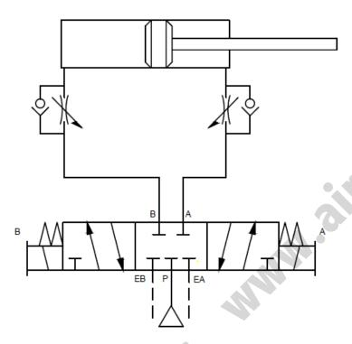
This is the type of valve most frequently selected to stop or jog an air cylinder. Be aware of the following when the valve is in mid position:
